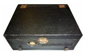
General view of French 33X 'suitcase' set with front lid closed. Note the round opening with push button which was used as an emergency Morse key.
